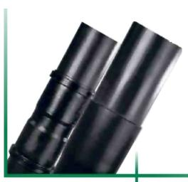
There is no need to use connectors while using pipes with push fit sockets (with the exception of those with a 3.7 millimetre-wall). In this case, leak-proof status is achieved in a similar fashion to that utilizing the coupler without rubber seals, thanks to the tapered shape of the socket and the use of sealing greases and silicon.
